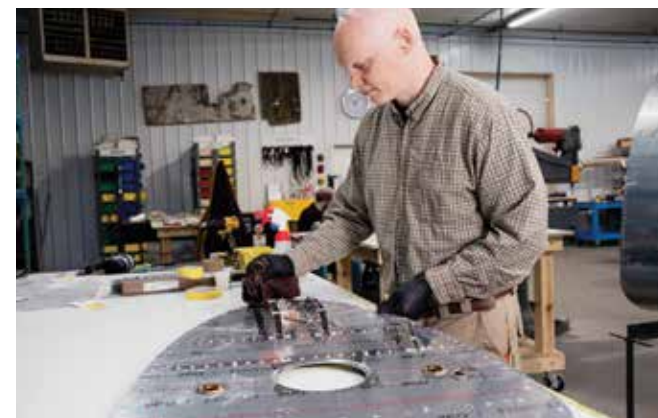
ABOVE LEFT: Brad and Paul work on fitting longerons. ABOVE RIGHT: Jacob works on the station 248 fuselage bulkhead. Station 248 is at the front of the tailcone assembly. The two brackets near the top of the bulkhead are for elevator cable pulleys.
