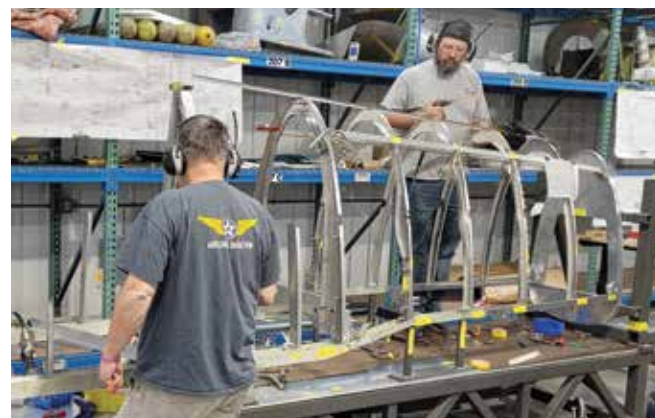
ABOVE LEFT: Brad and Paul work on fitting longerons. ABOVE RIGHT: Jacob works on the station 248 fuselage bulkhead. Station 248 is at the front of the tailcone assembly. The two brackets near the top of the bulkhead are for elevator cable pulleys.
