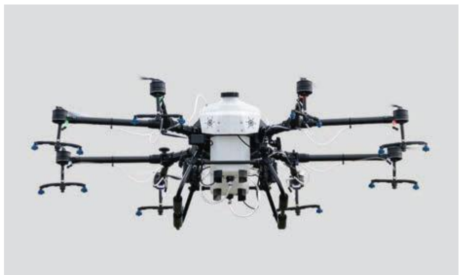
HYLIO AG-230 is 8 gallons and the company also has 2.5-gallon, 4.5 gallon and 18-gallon UAS.
