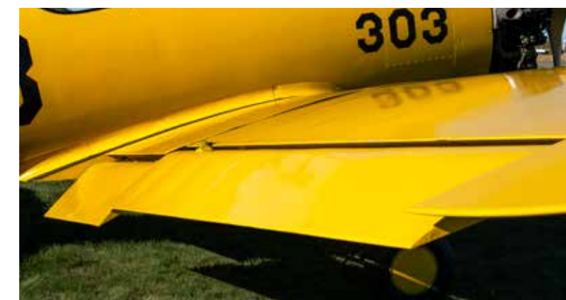
Clockwise from above: The Timm's main gear are spaced widely and aid in the trainer's docile handling on the ground. ■ Ed Newberg stands next to N69822, the N2T-1 he and son Dustin purchased in 2012. ■ The N2T-1's flaps, inboard of the aileron here, are hydraulically powered. It's an odd feature Newberg says, adding that he doesn't understand why Timm chose to actuate the relatively small flaps with hydraulics. ■ As a nod to O.W. Timm and the distinction of him being the first flier to take Charles Lindbergh aloft, Newberg's mechanic Jay Anderson embedded authentic Lindbergh coins in the N2T-1's front and rear cockpit instrument panels, between the airspeed and turn and bank indicators. (Photo by Ed Newberg)
