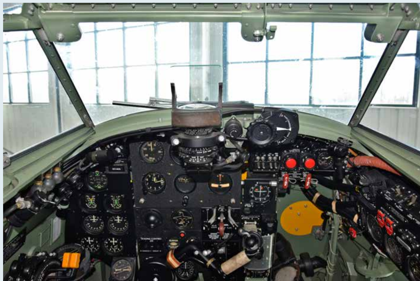
ABOVE: Spalding's "office." The Mossie is effectively a single pilot airplane. Flight controls and most of the engine management controls fall easily to hand but certain actions, like feathering an engine or opening/closing the Merlin's cowl flaps, require the pilot to reach across to the right side of the instrument panel.
