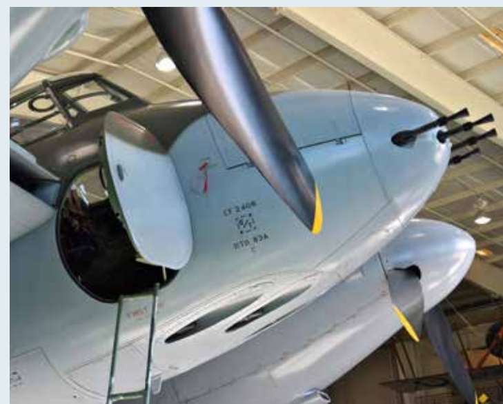
BELOW: Entry to KA114 is through the door that opens on the lower right side of the Mosquito's nose. The airplane's fragile integral ladder is extended here. Up on the nose are two rows of guns: four .303 Browning machine guns above with four 20 mm Hispano Mk. II cannon in the chin. (Photos by Justin Fortier)
