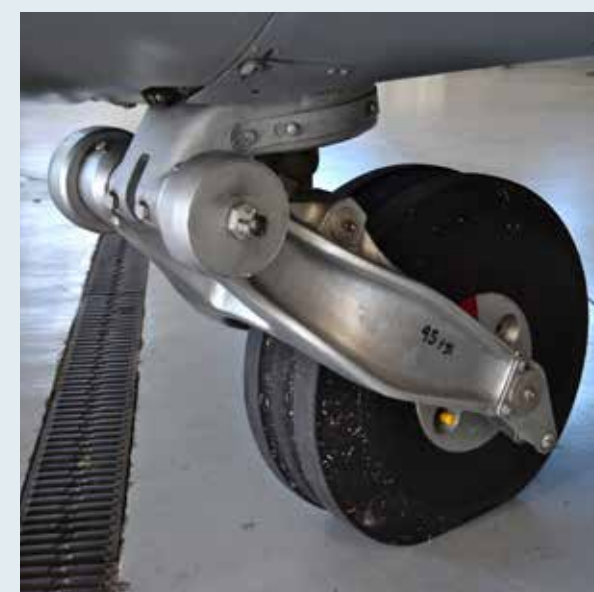
ABOVE: The Mosquito's tail wheel doesn't lock, Spalding says. But it does have a self-centering action that helps the twin engine fighter-bomber to track straight on the ground.
