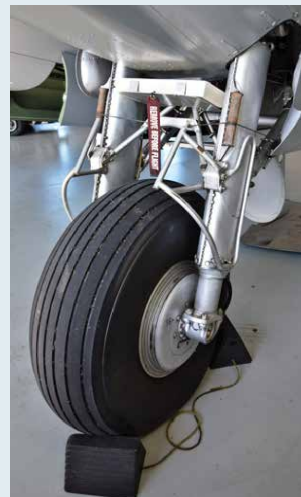
BELOW: The main gear must be inspected carefully before flight and taxied with care, Spalding notes. Side loads imparted by turning the aircraft too abruptly can damage the mains. (Photos by Justin Fortier)
