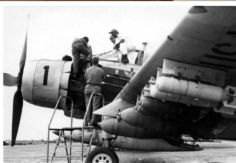
Right: An A-1E armed and ready to go at Qui Nhon Air Base, loaded with a mix of 100-pound white phosphorus bombs, 250-pound general purpose bombs, and either 750- or 500-pound GP bombs. (Photo courtesy Tom Dwelle via Byron Hukee)
