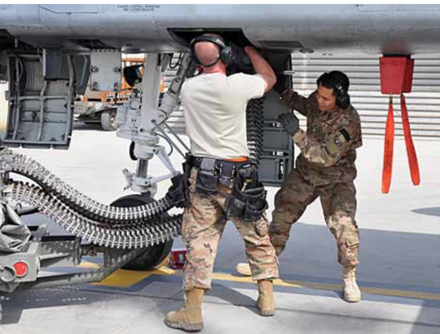
ABOVE: Munitions systems airmen load foot-long 30 mm slugs into an A-10's GAU-8/A Gatling gun at Bagram Air Base, Afghanistan. (U.S. Air Force photo via DVIDS)
