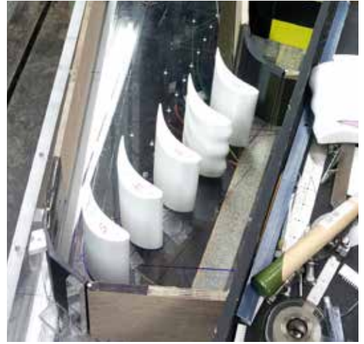
▲ A wavy blade design based on a harbor seal whisker was tested among reference blades in a transonic wind tunnel at NASA’s Glenn Research Center. Test blades are geometrically larger than real turbine blades to better characterize the flow physics. Vikram Shyam
