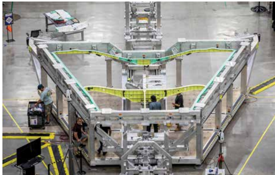
▲ NASA's X-59 Quiet SuperSonic Technology airplane, including parts of its wing, is under construction at the Lockheed Martin Skunk Works factory in Palmdale, California. Lockheed Martin
