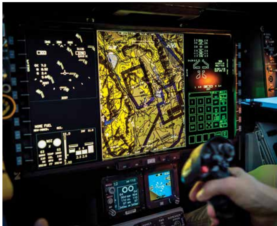
▲ The yellow display in this F/A-18 cockpit trainer is the situational awareness screen. The dark screen with white text in the upper left corner is the Advanced Targeting Forward Looking Infrared, or ATFLIR, display. Pilots report seeing strange objects on the displays.
