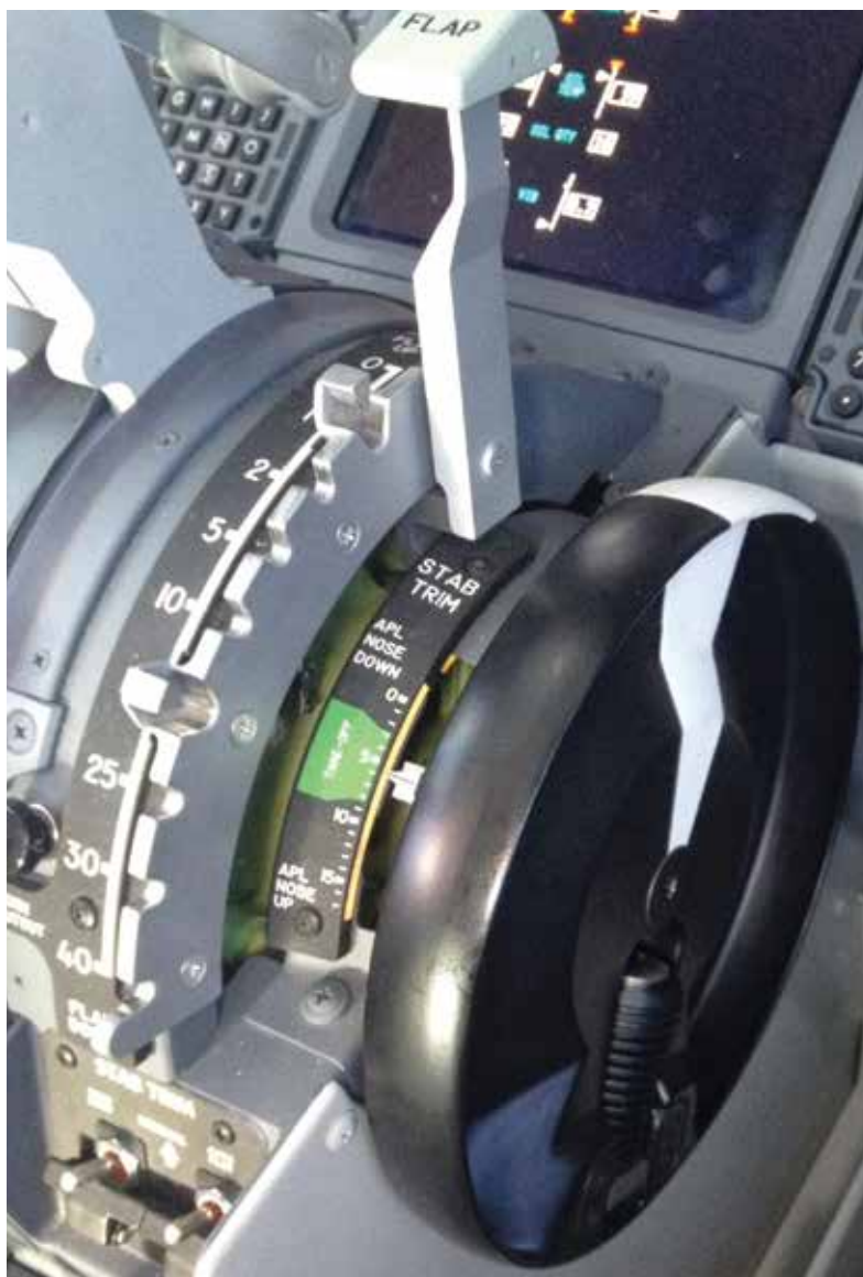
▲ A Boeing 737 MAX throttle trim wheel. The autopilot stab trim cutout switches are at lower left.
