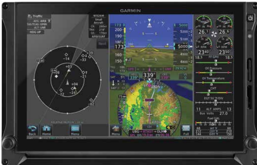
◀ ADS-B air traffic is indicated by white diamonds on the left hand side of this cockpit screen. A receiver picks up the signals and relays them to the G600 TXi display, which can be installed on single- and twin-engine general aviation aircraft. Garmin
