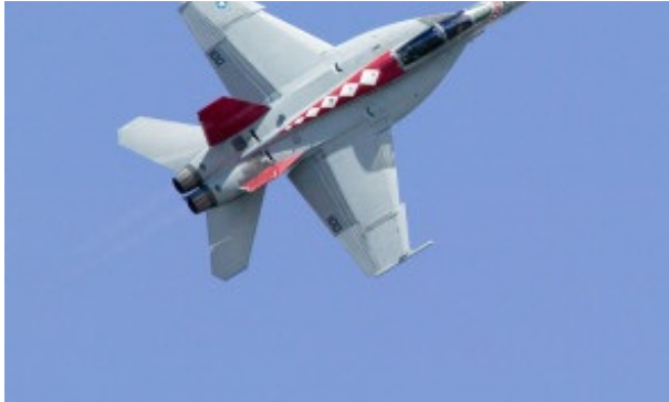
A Super Hornet is put through its paces. This second generation of Hornet, often called the Rhino, provides the airframe for the EA-18G Growler, often called the Grizzly. Boeing photo
