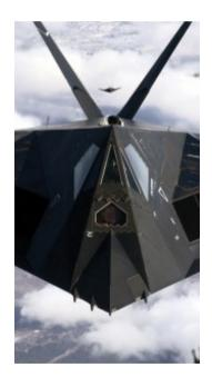
The F-117A Nighthawk was the world's first operational aircraft designed to exploit low-observable stealth technology. This
