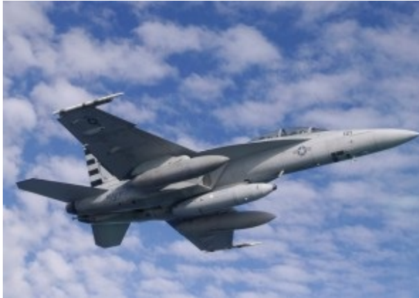
An F/A-18F Super Hornet flies with an infrared search and track (IRST) system integrated in the front section of the aircraft's centerline fuel tank during system flight testing. Boeing Company photo
