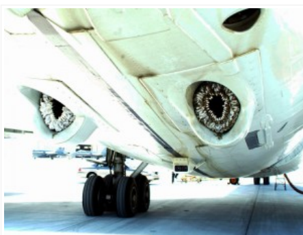
An Omega Air Boeing K-707 tanker aircraft showing the unique centerline aerial refueling system of the aircraft with its dual hose and drogue refueling gear stowed. DoD photo
