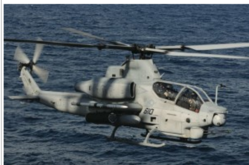
An AH-1Z Cobra helicopter assigned to Rotary Wing Aircraft Test Squadron (HX) 21, based in Patuxent River, Md., approaches the amphibious assault ship USS Wasp (LHD 1). The helicopter features a larger engine and has two more blades than the Cobra's original two, giving it more power and maneuverability. Wasp was chosen as the platform to evaluate the limits and capabilities of newer models of aircraft. U.S. Navy photo by Mass Communication Specialist 1st Class Rebekah Adler.
