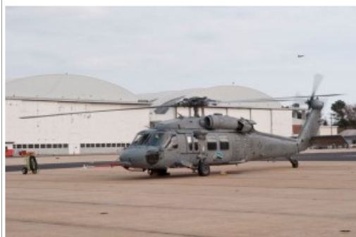
The Sea Hawk helicopter assigned to HX-21 Blackjacks carrying out the testing of a 50/50 Camelina seed-based biofuel blend spools up at Naval Air Station Patuxent River, Md. Testing has so far shown no significant performance differences between the fuel and standard jet fuel. U.S. Navy photo.
