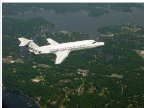
Northrop Grumman's BAC 1-11 in flight over central Maryland. This aircraft is being used to test the radar and DAS that will be employed by the F-35. Northrop Grumman photo.
